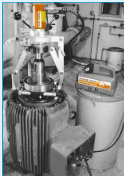
SGH153CR with a bearing pulling attachment was used to take a bearing off a utilities well pump motor.
